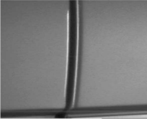
Fig. 2. A gap on the outer surface of a vehicle, which is highlighted for measurement purposes.
