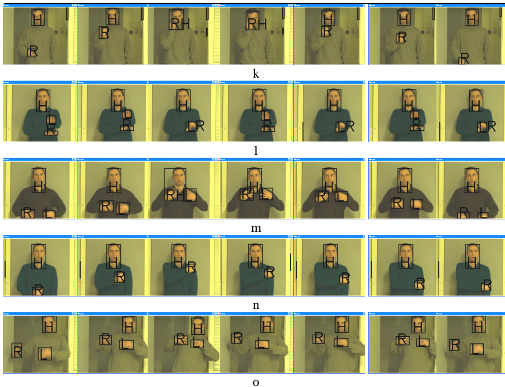
Fig.2 (i)-(o) The extraction of mid-level semantics from skin regions in sign language videos for the words: (i) amount (j) annoy (k) ashamed (l) afternoon (m) anger (n) anger, (o) assume
