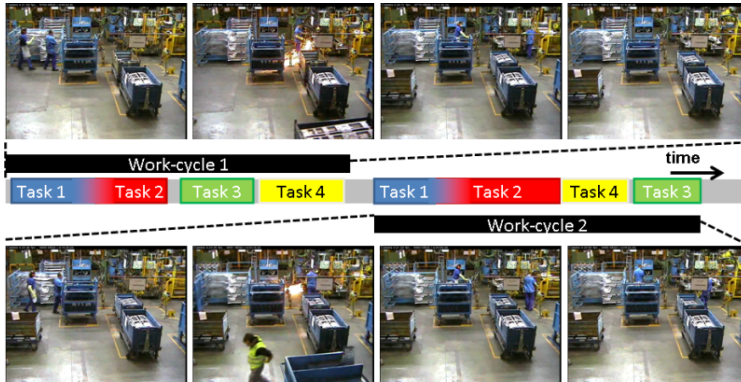
Figure 1: Example of an industrial scenario: a workflow consists of several tasks of different length, which can be permutable (e.g., tasks 3 and 4 in this example), and the scene may present irrelevant motion and occlusions.
