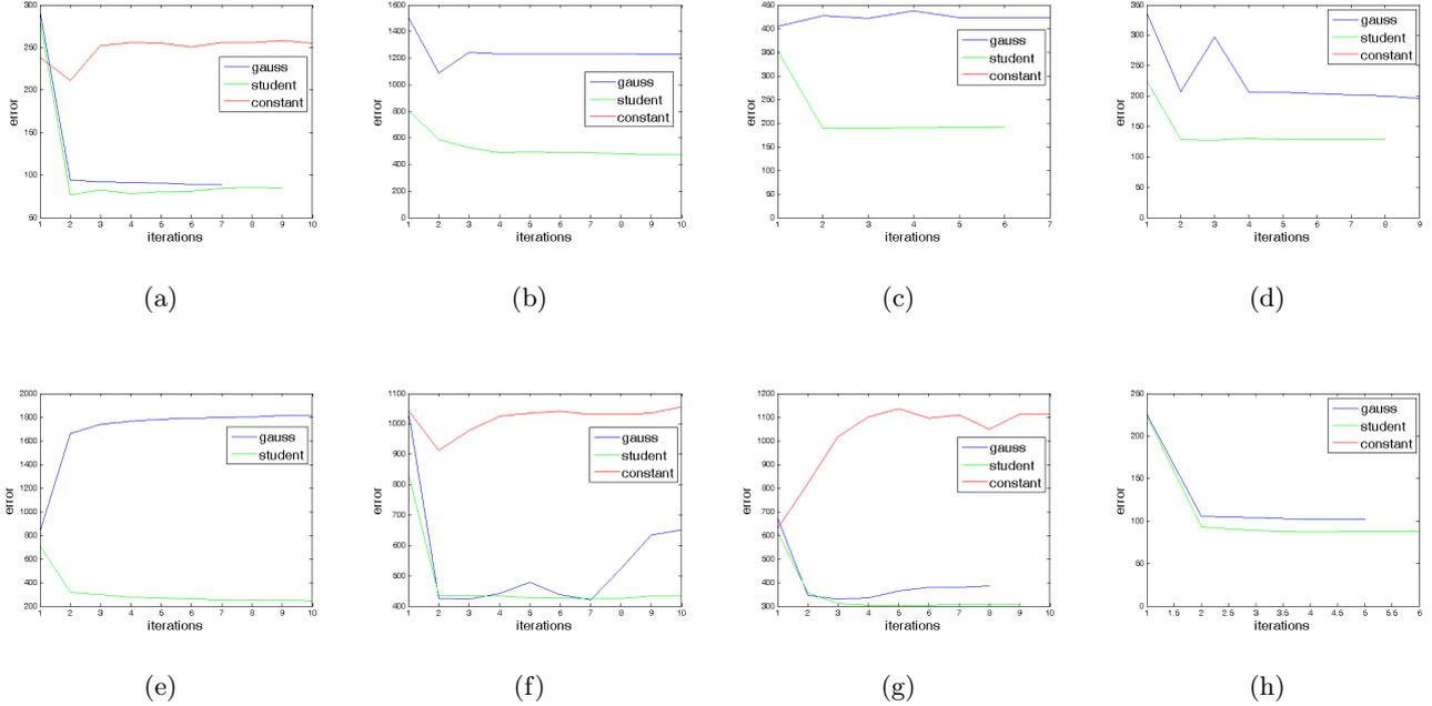
**Figure 4: Typical loop cases demonstrating convergence and accuracy of the proposed Student- $t$  based model, of the conventional Gaussian as well as the constant motion model. The constant model in several cases failed to converge. The error is calculated from (21) and the measurement units correspond to cell distance in the grid.**
