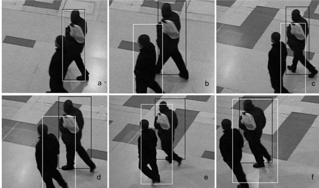
Fig. 5. Tracking Results - PETS Sequence: White PF, Black PM, 100 particles, frames 1,15,30,45,60,75.
